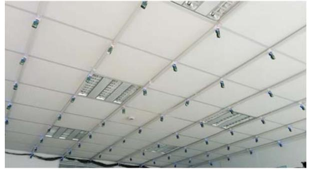
Fig. 4: Indoor testbed consisting of 80 TelosB nodes.
