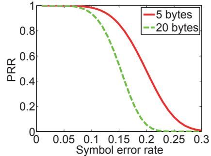
**Fig. 3: The SER-PRR curves with different packet lengths.**
