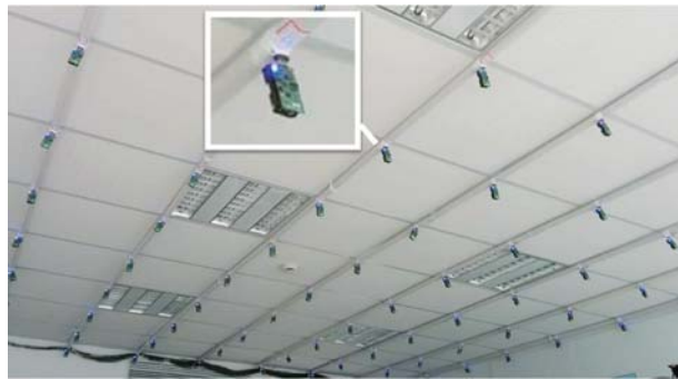
Fig. 7: The 8 \times 10 testbed with TelosB/TinyOS nodes.
