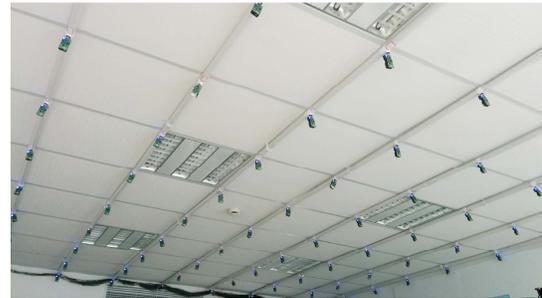
Fig. 9. The test-bed with 80 TelosB nodes.
